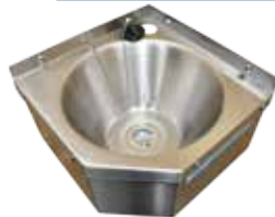
Wall Mounted Corner Handbasin Code: HBC $94 Outer size 265 x 265 x 165 high, 25mm splashback. Bowl size 230mm diameter x 120mm deep. Bowl Holds 2.5 Litres. FREE Sink waste drainer included.
