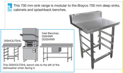
Accommodates 3 x 500 mm (19 3/4") commercial dishwasher racks. FRONT SIDE 800 130 150 20 mm \_ 50 180 100 dishwasher lip 1050 515 170 ь 170 250 115 TOP 700 550 780 20 mm **COMPONENTS** dishwasher lip Splashback 150 mm (high), 130 mm (deep) Welded sockets 2 mm Stainless legs 40 mm x 40 mm **Dishwasher racks** To fit 500 x 500 mm racks x 3 It is important that your Adjustable feet stainless steel is kept clean to extend the lifetime of the product.
